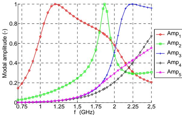
Fig. 2 Modal amplitudes  $1/|1+j\lambda_n|$  of the dual-PIFA structure. The frequency of interest is 2 GHz.
