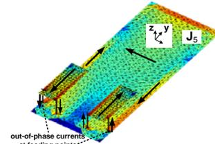
Fig. 5. Distribution of the characteristic current  $J_5$  at 2 GHz
